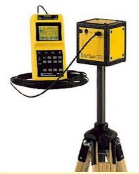
FIG. 6. Electromagnetic field analyzer and its electric field probe
